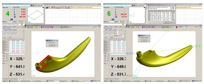
Having aligned to the CAD model, any points taken in any measured feature will now appear in the CAD window. These points will be displayed as a colour-coded dot on the model, and can either have a line leading to a box showing the error of the measured point, or alternatively the length of the attached line can be proportional to the error. In this way it is easy to visualise the distortion of a surface relative to the theoretical model.
