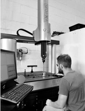
Although the capabilities, accuracy and speed of Coordinate Measuring Machines (CMMs) can often be similar, the diverse nature and the varied operating characteristics of CMM manufacturers' software means that the deciding factor for potential purchasers is frequently the CMM's software. This was the case when [Wrate Engineering Co](#) recently purchased a CNC version of Aberlink's popular [Axiom too CMM](#).
